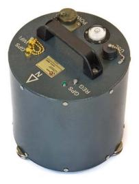
**CME-6011ND** is a digital 3component low-noise broadband seismometer with a force feedback. A bandwidth of up to **30 sec** provides recording of the remote seismic events.
