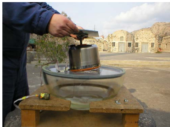
Fig 2. The CME4211-OBS installation into a deep-water sphere. Photo by courtesy of GeoPro GmbH, Germany
