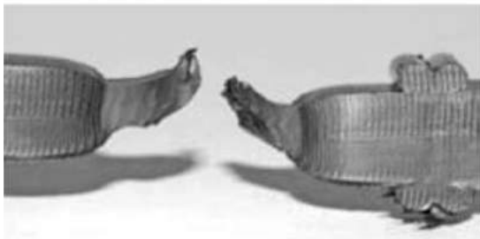
(b) Ductile Rupture Outside Fusion Interface
